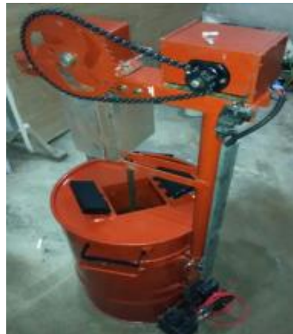
Figure 2: Stir Casting furnace
