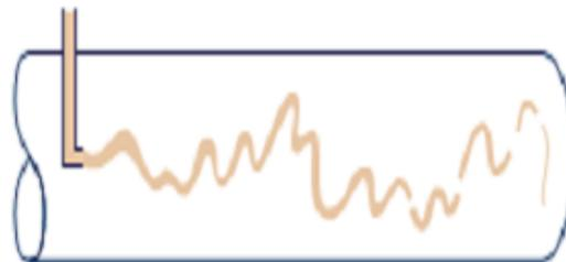
Gambar 2.23 Aliran Turbulen (Munson dkk, 2012)
