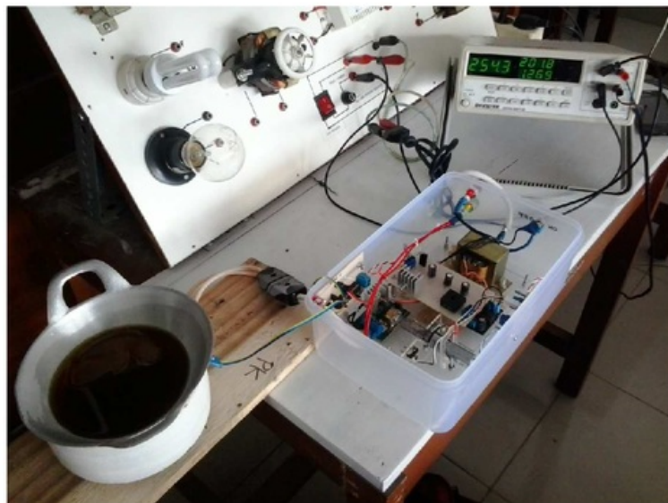
Figure 5. Automatic Batik Stove Design
